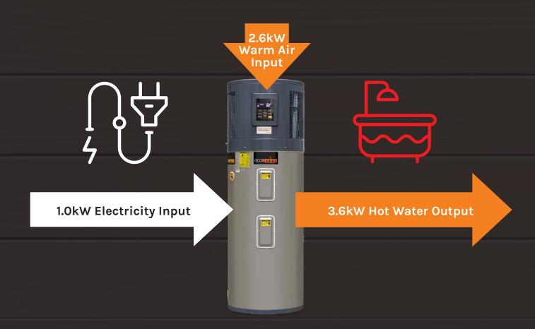
1.0kW Electricity Input + 2.60kW Atmospheric Heat Input = 3.60kW Hot Water Output\*
